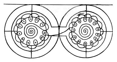
and fastened so that as it unwinds in one of the boxes it winds up the other in the second box. The clock is wound once a day, and as the running down of one of the spiral coils winds up the other the latter serves to run the clock during the night. Though it was described with much detail the mechanical working of it was not made clear, and hence we can only mention the ingenuity of the subconsciousness in constructing a plausible piece of machinery.
